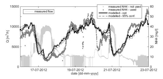
**Figure 12.** Model vs. monitoring data:  $NH_4$  concentration in the WWTP influent catchment Riool-Zuid between 16 July and 23 July. 'Double' dilution dips occur at 17 July around noon and 18 July around midnight and on 21 July at 2:00 a.m. and 12:00 a.m.
