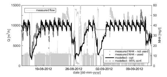
**Figure 15.** Gap filling with the influent model. Example for NH<sub>4</sub> in WWTP influent catchment Eindhoven.
