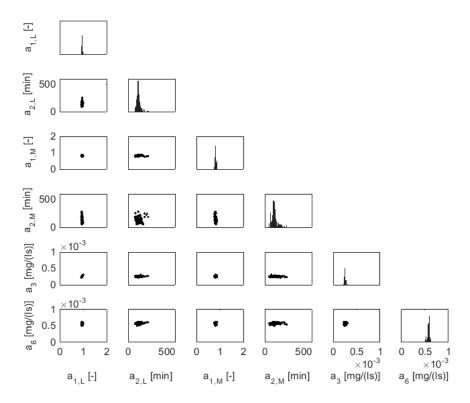
**Figure 7.** Posterior distribution of model parameters  $a_1$  to  $a_6$  for the NH<sub>4</sub> model for catchment Eindhoven Stad based on the second 50% of the iterations. The histograms represent the posterior distribution of individual model parameters and the scatter plots represent the relationships for various combinations of parameters.
