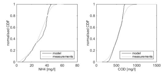
**Figure 9.** CDFs of model results and measurements for NH<sub>4</sub> and COD in WWTP influent for the Eindhoven Stad (ES) catchment.
